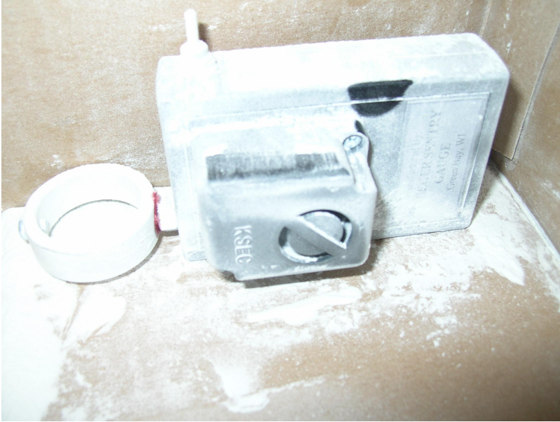
Figure 2. This is the unit after dust-proof testing. Test consisted of about 2 table spoons of Baby Powder in a vacuum tight box. The box was shaken several times while being held at a pressure lower than atmospheric pressure with a vacuum pump.
